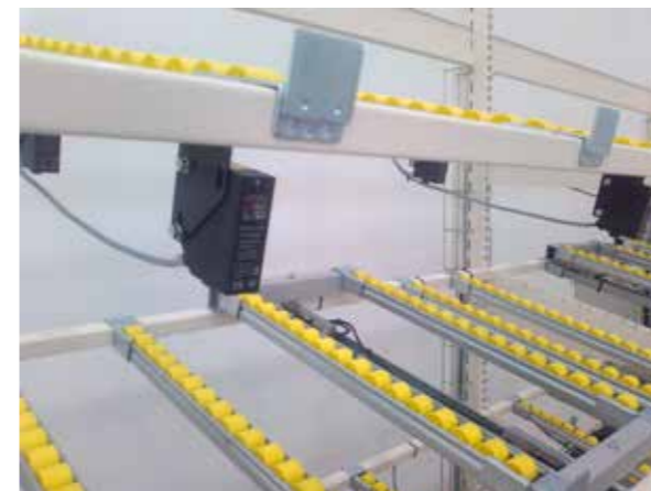
Photocells in the Inventory Control Module
