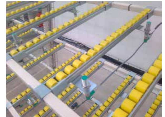
Inductive and capacity sensors in the Inventory Control Module
